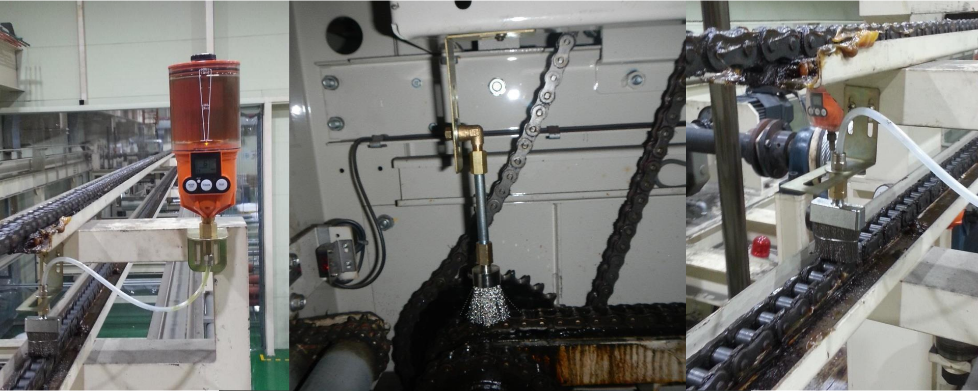
Pulsarlube OL500 multi lubrication with brush application.
